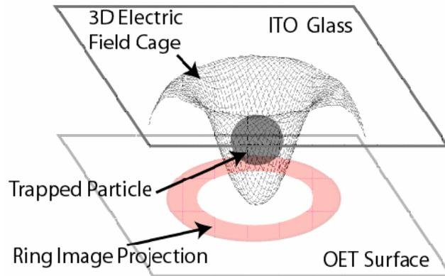
Fig. 2. Electric field distribution for a single-particle ring trap.
